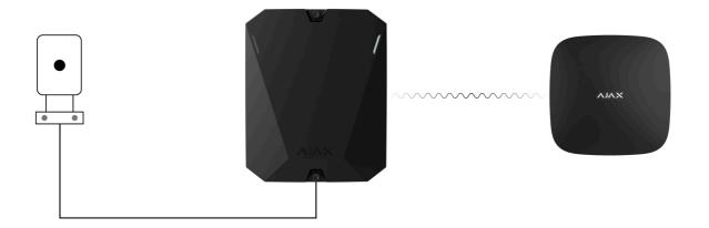
MultiTransmitter can be used to connect alarm and auxiliary request buttons, indoor and outdoor motion detectors, as well as detectors that track opening, vibration, glass breaking, fire, gas and water leakage, etc.
